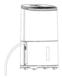
**Step 4:** Insert the water tank back into the dehumidifier.
