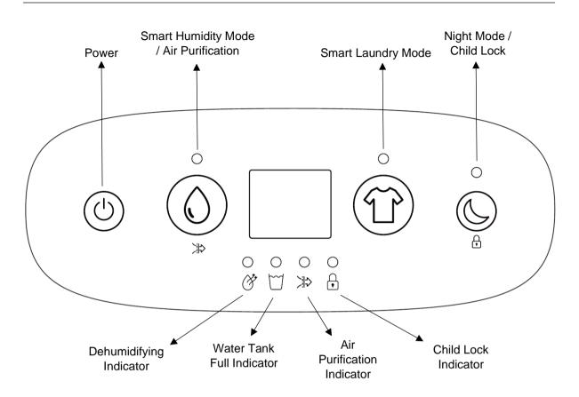
When the dehumidifier is first plugged into the mains it will bleep once, no lights will appear on the control panel. All buttons on the control panel only require a short press. Press the buttons firmly and quickly
